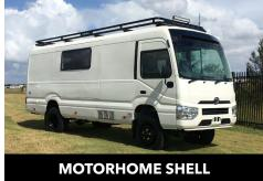
Toyota Coaster has always been the benchmark for medium sized people movers and Bus 4x4 has made it even better with its proven 4WD conversion kit\*. In addition to converting the Coaster into Full Time 4WD with high and low range capabilities, the body is raised to 215mm and modifications made to the drive-train, suspension and braking systems. All of the Coaster's excellent safety and comfort features are retained.
